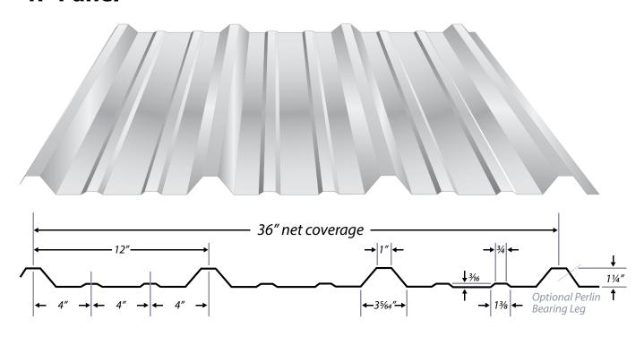
"R" Panel is a multi-use wall and roof panel used primarily in pre-engineered metal building applications.
