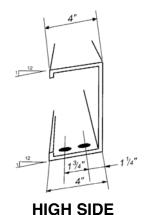
struts are available in the same sizes and gauges as standard eave struts. When ordering, please request double slope.
