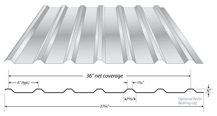
"U" Panel is an exposed fastener wall and roof panel that is mainly used as a liner or partition panel.
