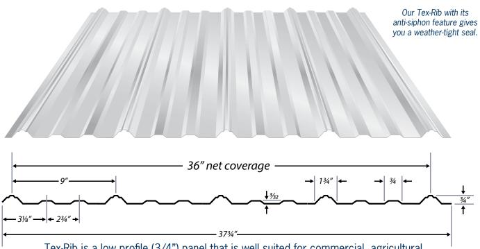
Tex-Rib is a low profile (3/4") panel that is well suited for commercial, agricultural and residential applications. Tex-Rib can be installed on as low as a 1:12 pitch if sealant is used on the sidelaps. If not, a 3:12 pitch is recommended.
